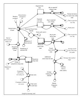
Figure 20 SFD of tram sub-model
