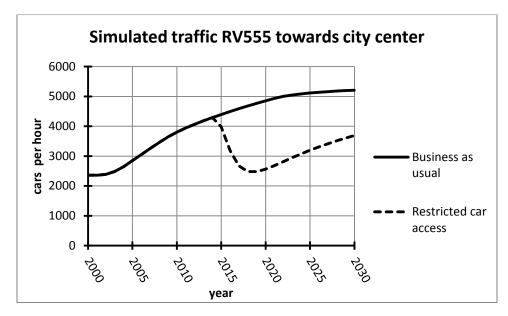
Figure 26 Effect of restricted car access simulated traffic RV555 towards city center
