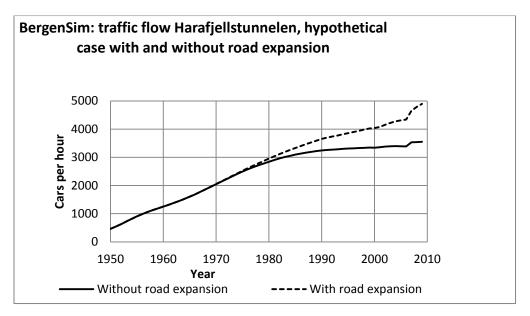
Figure 36 Importance of road construction in a historical perspective
