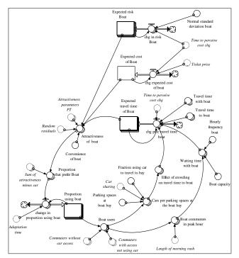
Figure 19 SFD of boat sub-model
