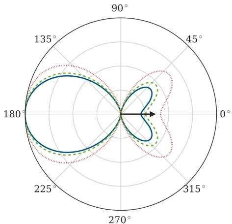
FIG. 6. (Color online) Angular distributions for double ionization with equal energy sharing  $E_1 = E_2 = (2\omega - I_p)/2$ . The arrow indicates the fixed direction of the first electron. Solid (blue) line:  $E_0 = 1$  a.u. Dashed (green) line:  $E_0 = 10$  a.u. Dotted (red) line:  $E_0 = 20$  a.u.
