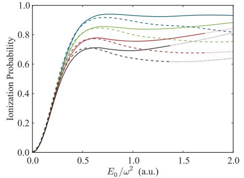
FIG. 3. (Color online) Ionization probabilities for a constant pulse duration of  $2\pi$  a.u. The lines correspond to laser frequencies of  $\omega = 4, 6, 8,$  and  $10$  a.u. from top to bottom, or equivalently pulse lengths of 4, 6, 8, and 10 cycles. The solid lines are the full calculations. The dashed lines are the IE calculations. The dotted parts of the curves indicate where relativistic (nondipole) effects may influence the results.
