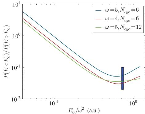
FIG. 8. (Color online) Ratio of slow to fast electrons for the double-ionization process, shown for different pulse frequencies and durations, and plotted as a function of  $\alpha_0$ . The blue bar indicates the region where the corresponding double-ionization probability is maximum, where stabilization sets in.
