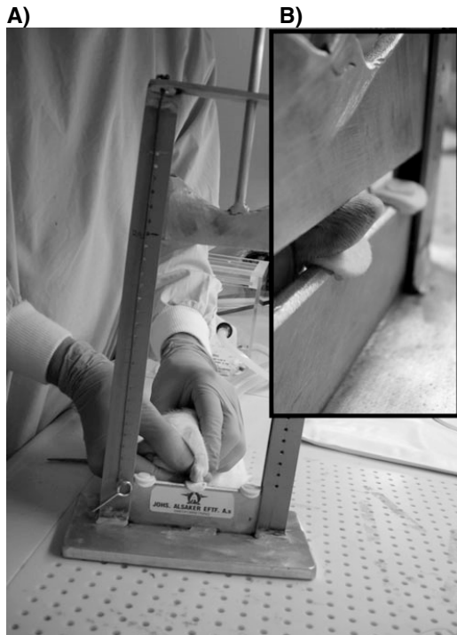
Fig. 1 a Mini guillotine with rat positioned for Achilles injury. b (insert) Close-up of the tendon crush location
