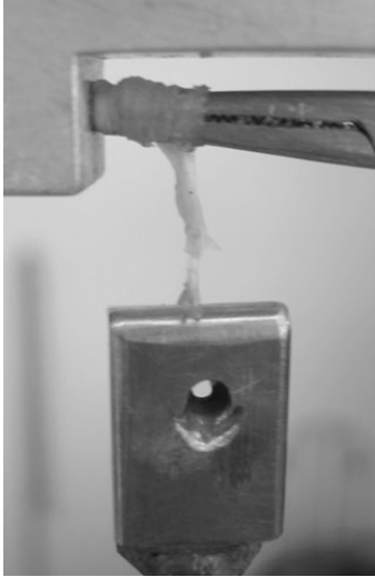
Fig. 4 A rat Achilles tendon at the moment of rupture during UTS testing
