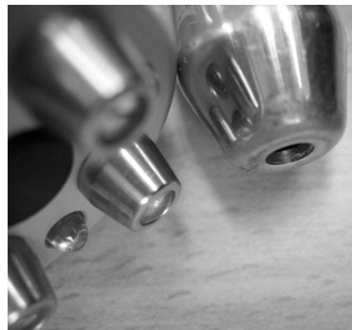
FIG. 3. Laser probe tip, the 904 nm laser with a protruding lens (left), and the 810 nm laser with a folded up lens (right).
