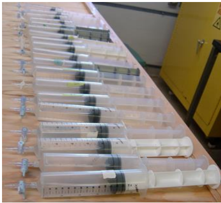
Figure 6. Water samples with He headspace gas ready for gas chromatograph analysis. Photo by Tamara Baumberger 2008.
