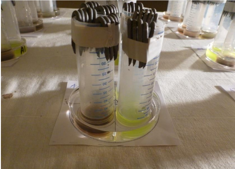
Figure 3 Combination B sedimenting while the Falcon tubes are weighed down using bent nails.
