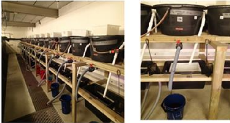
Figure 2 Host fish was kept containers with 90L of water during the harvest. The fish were kept in dark tanks to prevent the fish from eating the decysted young of the year mussels. When the glochidia matured and decysted from the fish, they were transported, using a pipe system, onto a sieve with a mesh size of 200µm placed below the containers (photo: Per Johan Jakobsen).
