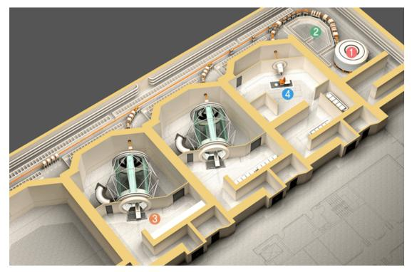
Figure 2-5: Schematic overview over a proton therapy facility which displays 1) the accelerator, here a cyclotron, 2) the transport beam lines, 3) the treatment rooms with rotating gantry and 4) the treatment room with fixed beam. Image from (27).
