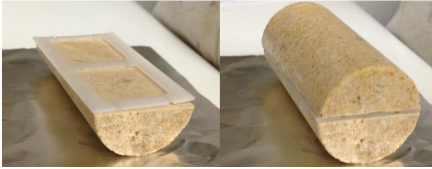
Figure 3.4 Fractured limestone core with spacer placed between the two parts. The chalk cores were cut in the same way and a similar spacer matching the length of the cores was used.
