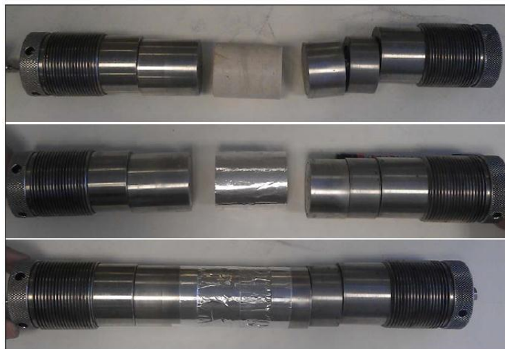
Figure 3.5 – Top: Core before and after it is wrapped in aluminum foil and attached to end pieces. Bottom: Core attached to the end pieces ready for montage to the core holder. Modified by (Haugen, 2012).
