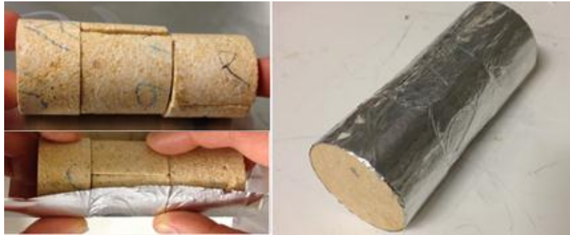
Figure 3.10– Left: Five parts before and after assembling them into the core holder. Right: All five cores put together and wrapped in aluminum foil to avoid CO 2 wearing out the sleeve and to keep it inside the system. The core was attached to the end pieces as shown in Figure 3.6.
