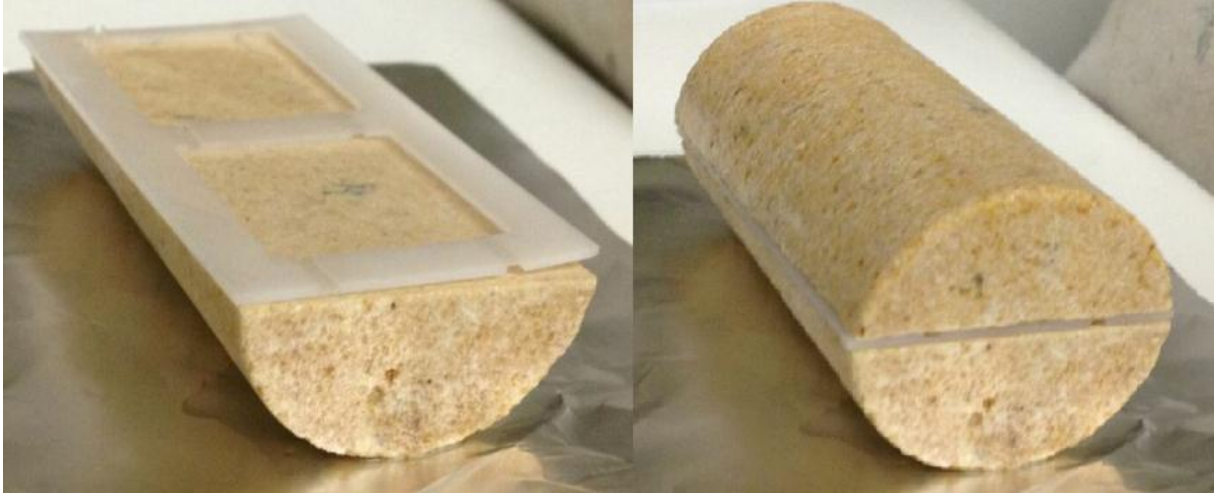
Figure 3.2 POM spacer used in experiments to maintain a constant fracture aperture.
