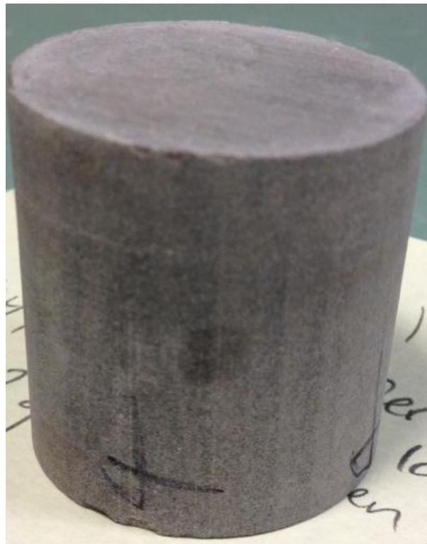
Figure 3.1 Reservoir shale core plug used for experimental test in this thesis.
