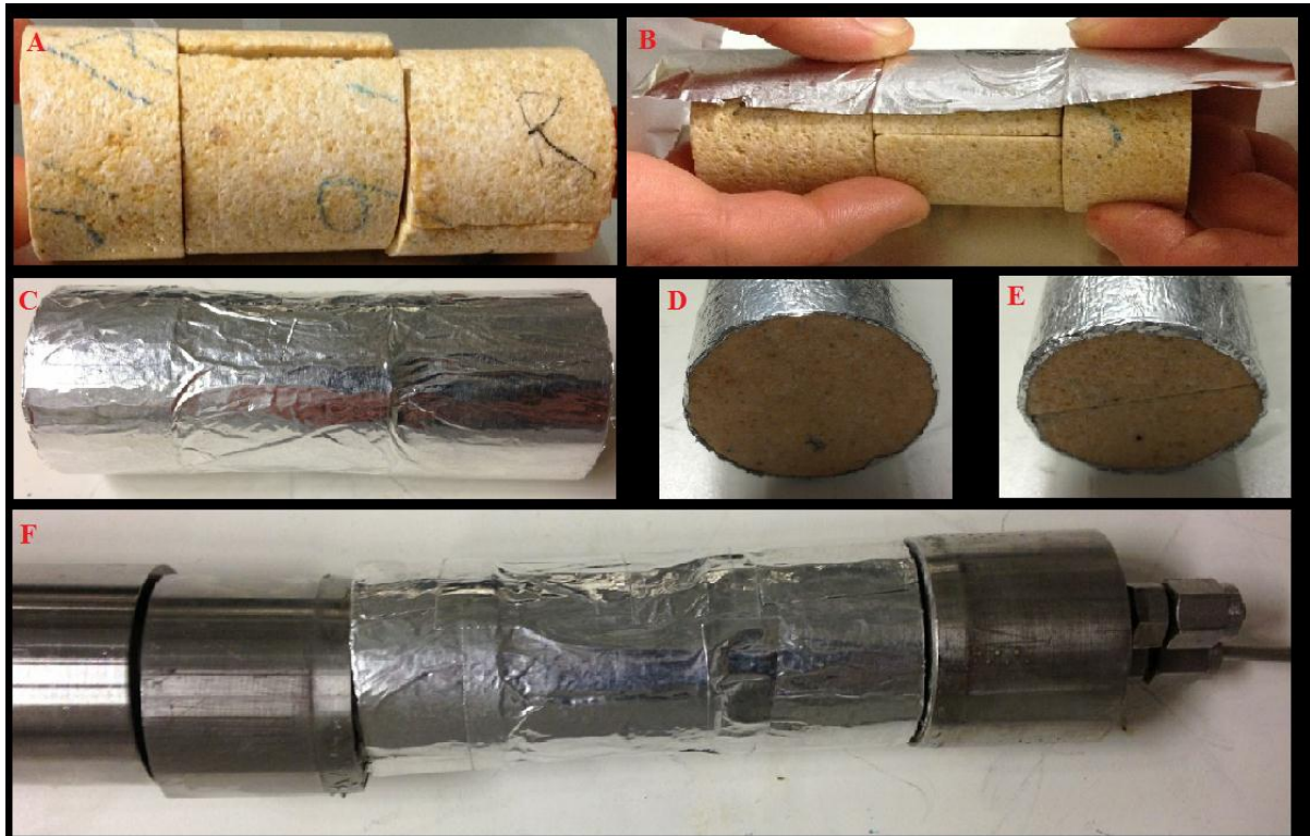
Figure 3.7 Preparation of the cores prior to experiment. The whole core piece was placed closest to the inlet, followed by a core piece with vertical fracture orientation and a core piece with horizontal fracture orientation.
