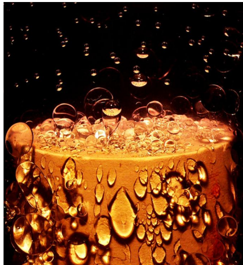
Figure 10: A chalk core surface during imbibition in mature gel. Oil drops were captured in gel for a long period of time, and the saturation could appear to be static for hours at a time.
