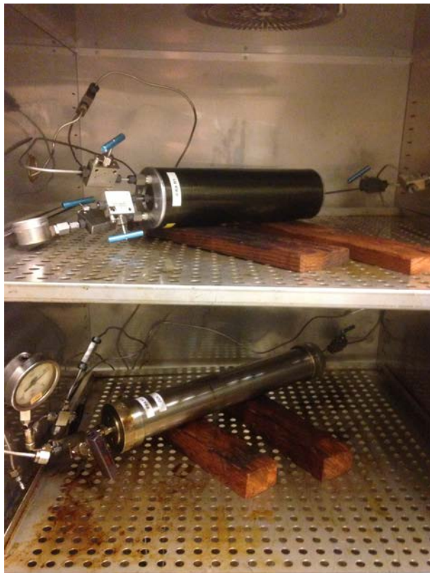
Figure 4.4: Cores in heating cabinet
