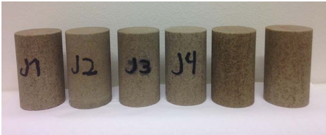
Figure 4.1: Berea cores used in the experiment, C1 and C2 are the two cores to the right
