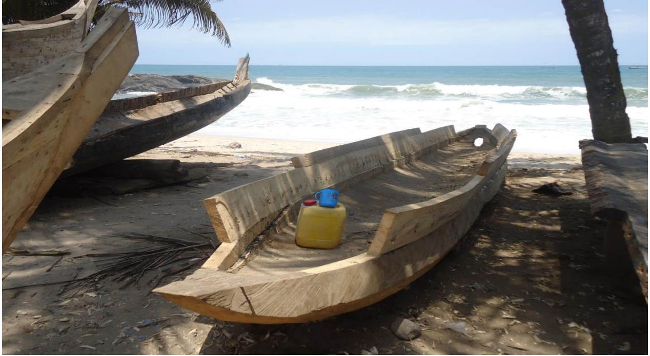
Photo 6: The base of the canoe which is being expanded into a complete canoe
