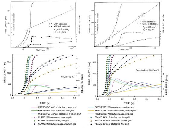
**Figure 6** Experimental (above) and simulated (below) pressure rise and location of flame front as function of time for flame propagation with and without obstacles in 6.2 % methane-air (left, FLACS simulations) and 550 g/m<sup>3</sup> cornstarch-air mixtures (right, DESC simulations) at an ignition delay time of 319 ms; experimental results from Pu (1988). The legend below the plots applies to the simulated data.
