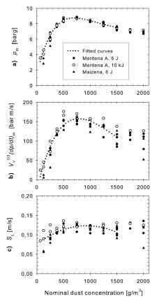
**Figure 3** Experimental results for two types of dried cornstarch: **a**) corrected explosion pressure, **b**) size-normalized rate of pressure rise (maximum value corresponding to a  $K_{st}$ -value of about 150 bar m/s), and **c**) estimated laminar burning velocities.
