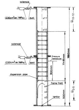
Figure 1 Schematic diagram of apparatus for explosion tests, from Pu et al. (1988). The closed tube is 0.19 meters in diameter and 1.86 meters long. It is filled with ring-shaped obstacles, and equipped with a piezoelectric pressure transducer and ionisation probes for measuring flame arrival. The ignition source was 0.6 grams of black powder, with total energy release about 1.75 kJ in 25 ms.
