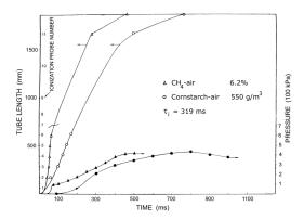
**Figure 2** Pressure rise and location of flame front as functions of time in 1.86 meter closed tube for mixtures of 6.2 % methane in air and  $550 \text{ g/m}^3$  cornstarch in air (from Pu, 1988).
