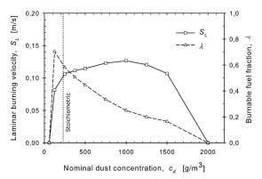
Figure 4 Laminar burning velocity and fraction of burnable fuel used as input to DESC; lower flammability limit estimated to 60 g/m<sup>3</sup>, upper flammability limit arbitrary set to 2000 g/m<sup>3</sup>.
