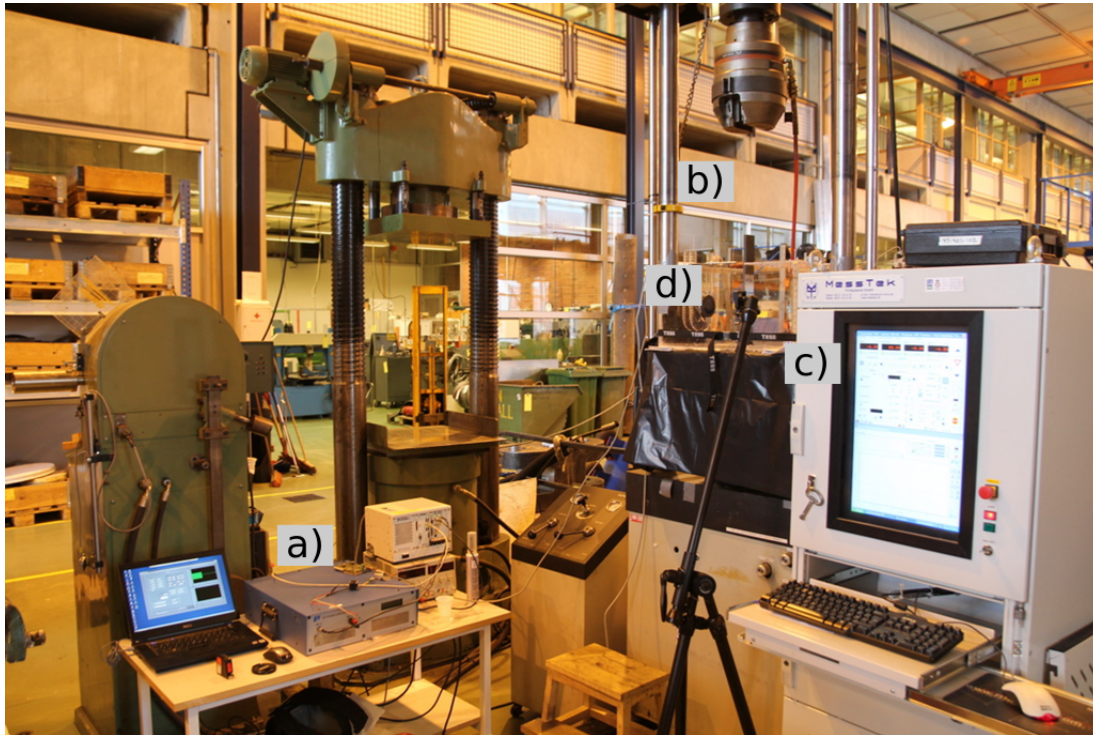
Figure 3.2: Experimental setup overview. a) acoustic setup, b) tension machine, c) control unit, d) water tank
