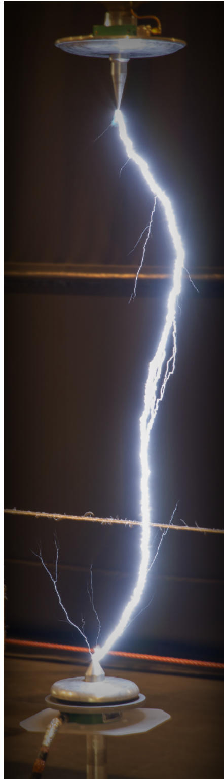
Figure 1.4: (Color) This photograph shows what a 1 meter long laboratory spark can look like. This photograph was taken by Lex van Deursen of the University of Eindhoven during our week of experimenting in January 2013.
