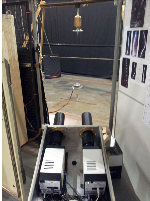
Figure 3.5: (Color) At the bottom, we see the two cameras pointed at the spark gap. At the middle and the top, we see the electrodes and the spark gap. On the left side of the photograph, we see part of the door of the cabinet.
