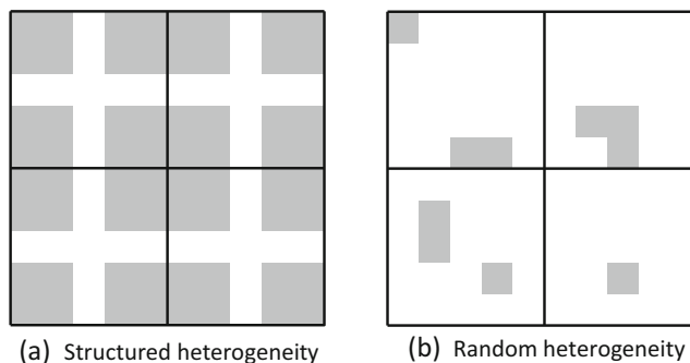
Fig. 5 Conceptual drawings of media with structured (left) and random (right) heterogeneities. White marks fine-scale cells with high permeabilities. Black lines indicate coarse cells. For the structured case, the low permeable area coincides with the interior of coarse dual cells
