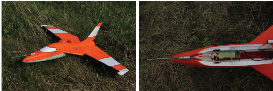
Fig. 1. Mounting of the turbulence system on the SUMO aircraft.
