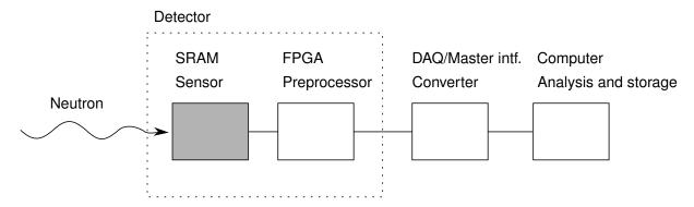
**Figure 4.1:** Overview of a detector system.
