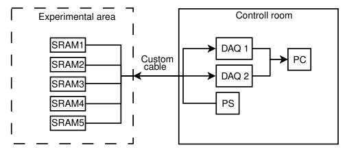
**Figure 5.9:** *Schematic setup of the the equipment used at CERF.*
