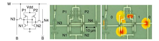
**Figure 3.1:** Image on left shows a standard 6T SRAM cell [16]. Center shows the same cell laid out in a 0.8 µm AMS BiCMOS technology, the spacing between transistors are exaggerated for testing purposes. Image on right shows the sensitive areas as mapped by a pulsed laser with energy from 10 pJ to 1193 pJ, darker color indicates higher sensitivity [17].
