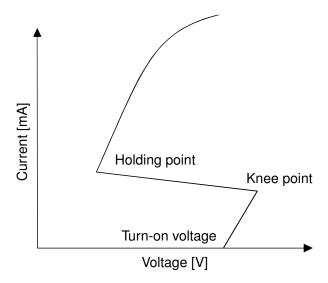
**Figure 2.4:** The latchup I-V characteristic [15].
