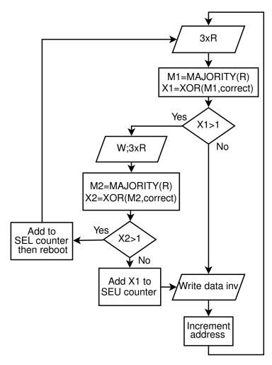
Figure 4.9: Flowchart for stuck bit mitigation.
