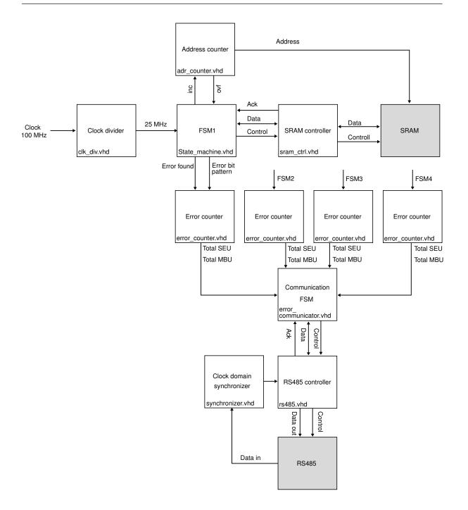
**Figure 4.5:** Block diagram of the firmware of the current detector. Boxes in gray are external components. The state diagram of the main finite state machine has the same flow as shown in the flowchart in figure 4.6.
