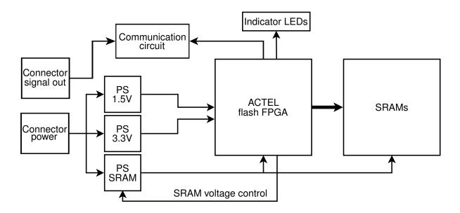
**Figure 4.2:** *Schematic overview of hardware for the detector.*
