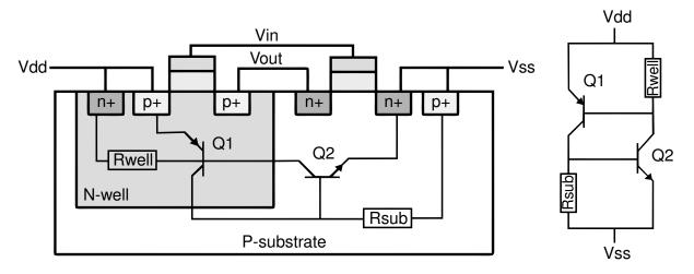
**Figure 2.3:** *PNPN parasitic structure in an N-well bulk CMOS inverter structure* [6].
