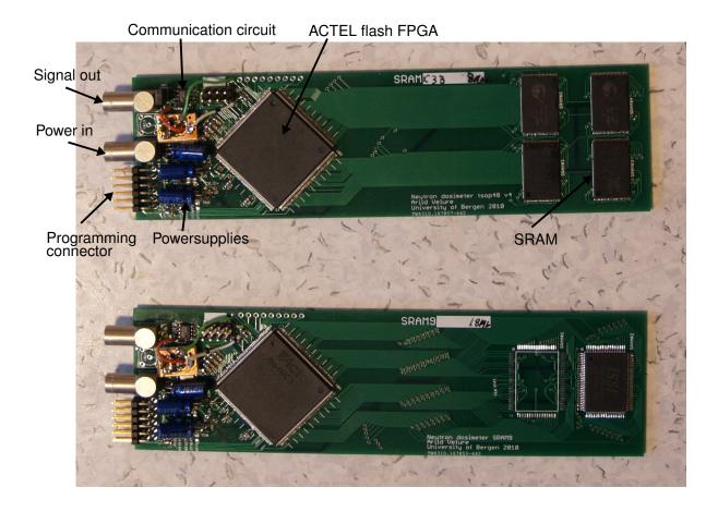
**Figure 4.3:** *Picture of two of the detectors.*
