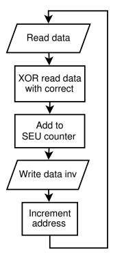
Figure 4.6: Simplified flowchart for SEU detection
