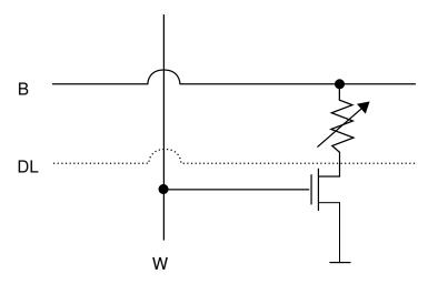
Figure 3.6: Schematic drawing of 1T MRAM cell.
