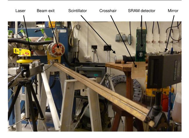
Figure 5.11: Overview of setup at OCL.
