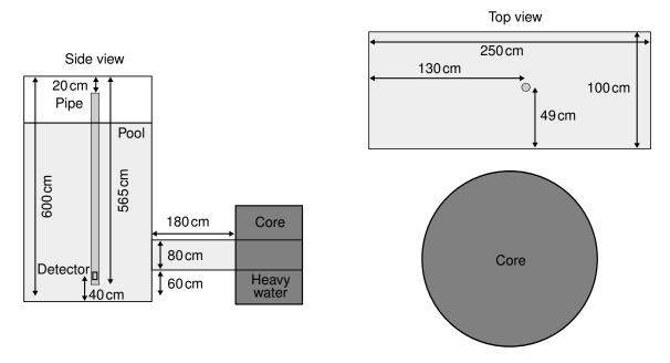
**Figure 5.14:** *Drawing of the placement of the detector in the pool. Not to scale.*
