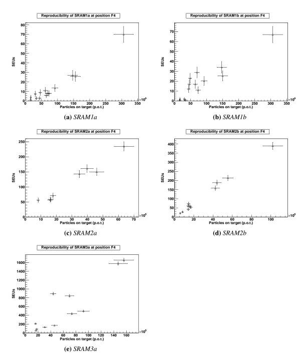
**Figure 6.4:** Reproducibility of SRAMs at position F4 at CERF.
