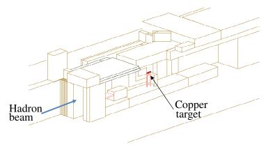
**Figure 5.4:** Layout of the experimental bunker at CERF as modeled in FLUKA [50].
