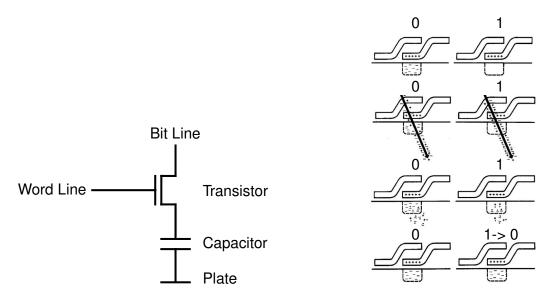
**Figure 3.2:** Schematic drawing of 1T DRAM cell [16].
