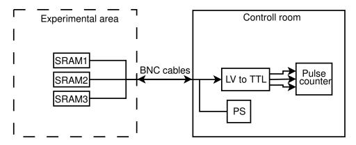
Figure 5.3: Schematic setup of the the equipment used at PTB.
