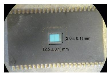
**Figure C.2:** The SRAM used for beam profile measurements. The top has been shaved off after irradiation to expose the die. During irradiation the short end was facing downwards.
