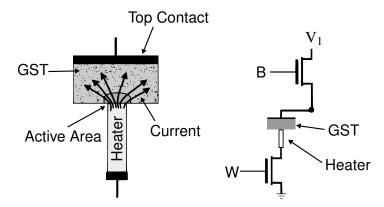
Figure 3.7: Schematic drawing of a PCRAM cell.
