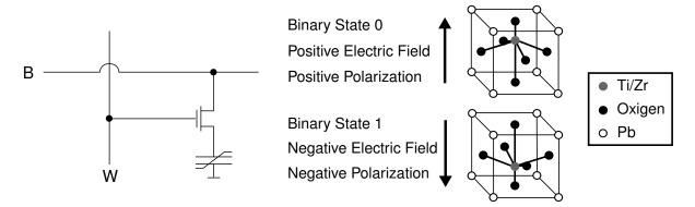
**Figure 3.4:** Schematic drawing of 1T FRAM cell [16].
