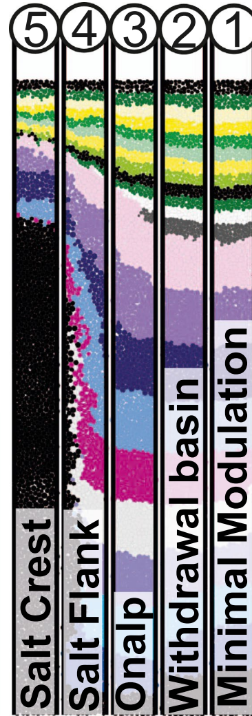
FIGURE 13 Halokinetic zonation scheme shown for M3. The model is divided into five zones, four of which experience some form of halokinetic influence. Minimal deformation zones 1 and all stratigraphy outside of it show virtually no modulation by salt diapirism. Halokinetic influence increases towards the diapir-cored high, and changes from minor thickness changes in the ‘withdrawal basin’ zone to onlap and abrupt pinch out in the ‘onlap’ and ‘salt flank’ zones. Thinned and reduced stratigraphy are observed over the diapirs crest. The table highlights that while stratigraphic trap quality may be greater closer to the diapir, reservoir thickness and quality are likely higher further from the diapir, showing a ‘trade-off’ exists for subsurface energy exploration and production. Similar zonation is possible for all models [Colour figure can be viewed at wileyonlinelibrary.com]
