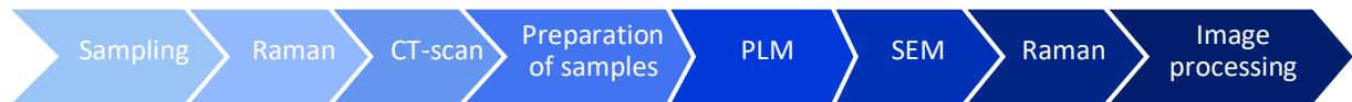
Figure 4.1: Flow chart of the methodology walkthrough. Step by step: sampling at the seafloor, Raman spectroscopy, CT-scanning, preparation of thick sections, petrographic light microscope (PLM), scanning electron microscopy (SEM), Raman spectroscopy, image processing.
