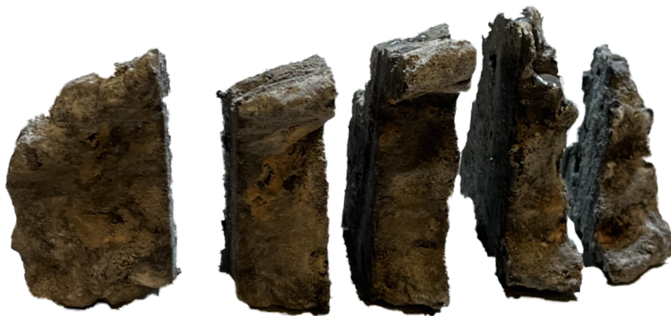
Figure 4.8: The Menorah chimney after cutting it in 5 pieces with the wire saw. The thick sections Menorah edge 1&2 are from the first piece from the left, Menorah middle 1, 2 & 3 is the third piece from the left, and Menorah top 1 & 2 is the last piece from the left. The thick sections of Menorah edge 1&2, Menorah middle 1,2 & 3 and Menorah top 1 & 2 are presented in the figures 5.16, 5.17 and 5.18 in Chapter 5.4.
