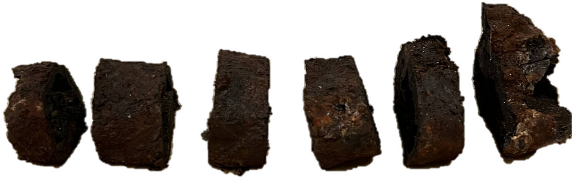
Figure 4.7: The Fåvne chimney after cutting it with the wire saw. The thick section Fåvne first piece is from the 1 piece to the left, whereas the Fåvne middle piece is from the third piece from the left is and the Fåvne third piece is from fifth piece from the left. The thick sections will be presented in Chapter 5.4 (Figure 5.13, 5.14 and 5.15).
