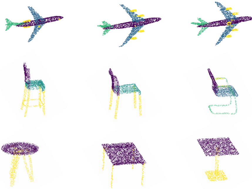
Figure 1.7: Point cloud samples from the ShapeNet dataset (Chang et al., 2015) Three different objects of airplane, chair, and table are visualized; colors represent the labels for part segmentation problem.
