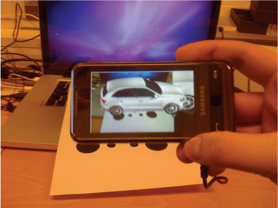
Figure 12: How a 3D car model might look using MAR with a newspaper. This prototype was used as an illustrative example to introduce HMAR to VG.
