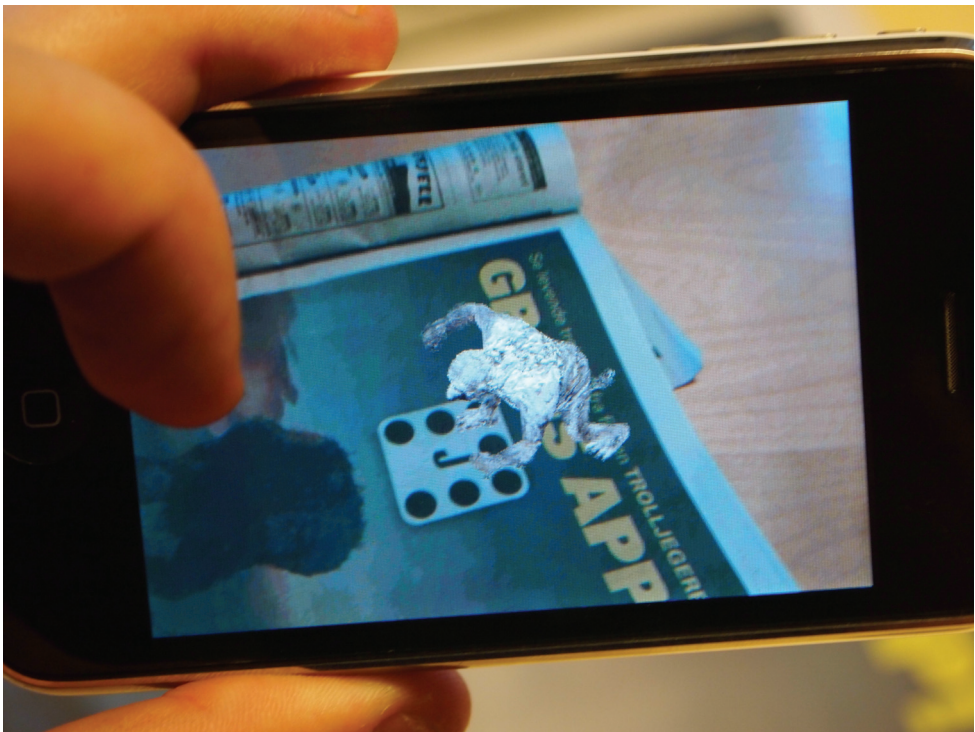
Figure 3: ARad augmenting a printed advertisement in a nationally circulated newspaper. The mobile display in figure shows an animated troll that allows for user interaction.
