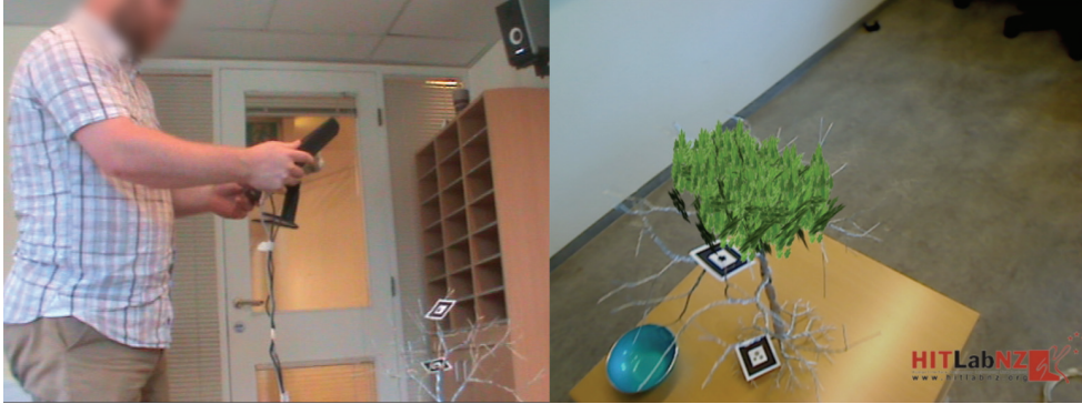
Figure 11: The tethered HMAR system used for evaluation of ArtAR. A tethered handheld display with a mounted camera was connected to a laptop running the system.
