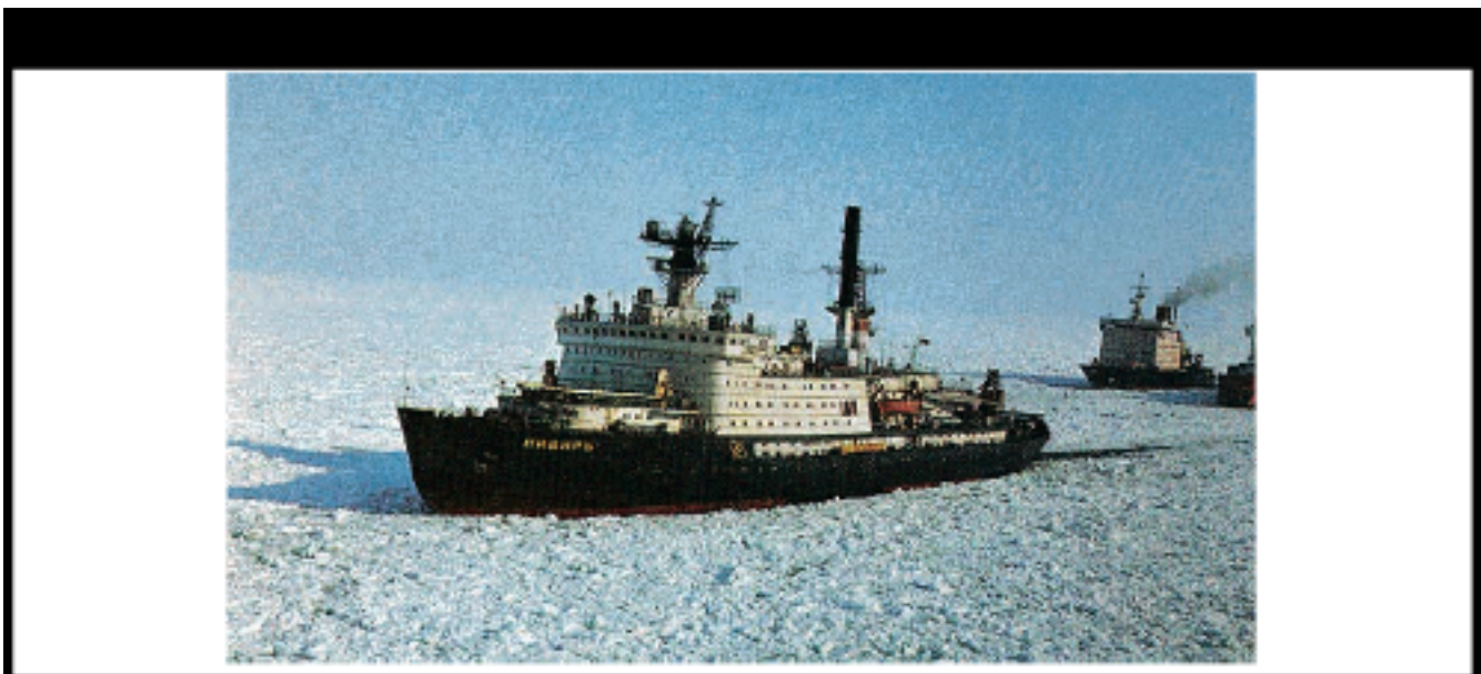
Figure 12 Picture of Russian nuclear powered icebreaker "Sibiria" leading a convoy of cargo vessels sailing through 2 m thick first-year ice in the Northern Sea Route. (Courtesy Murmansk Shipping Company.)
