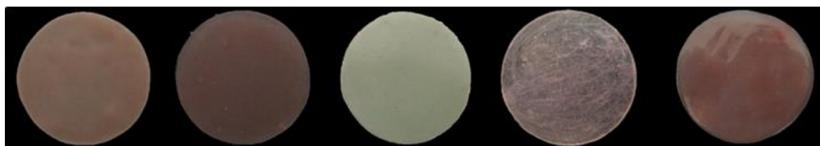
Figure 6. From left: Specimens of HIP, MRR, Palacos, Breflex, and Valplast.
