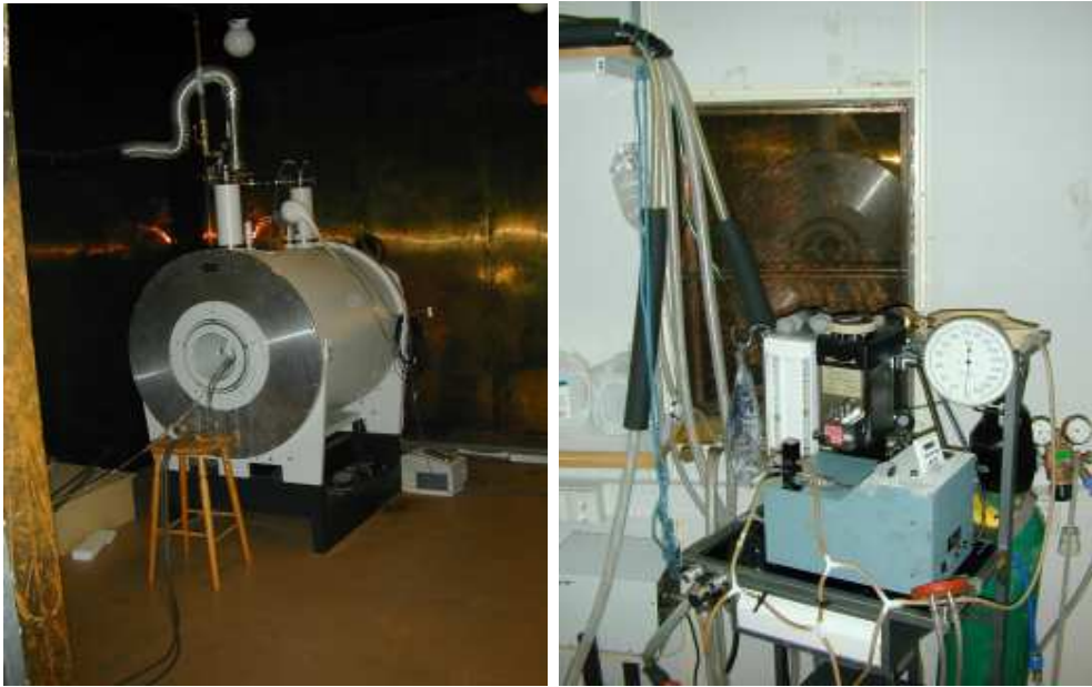
Figure 6.1.: The scanner and anesthesia equipment. The MRI scanner (left panel) being used was a 2.35 T Bruker Biospec Avance DBX-100 with 40 cm bore size. Right panel shows equipment by which animals were anesthetized.
