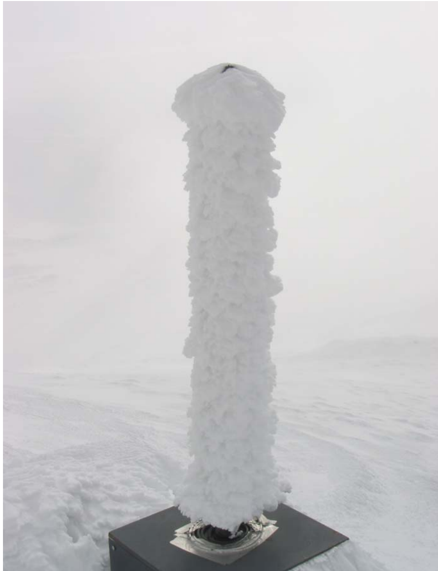
Figure 3.2. Ice scale with rotating 30 mm cylinder after icing incident at 1800 m a.s.l. at Mt. Gaustatoppen, 0925hrs April 2, 2003.
