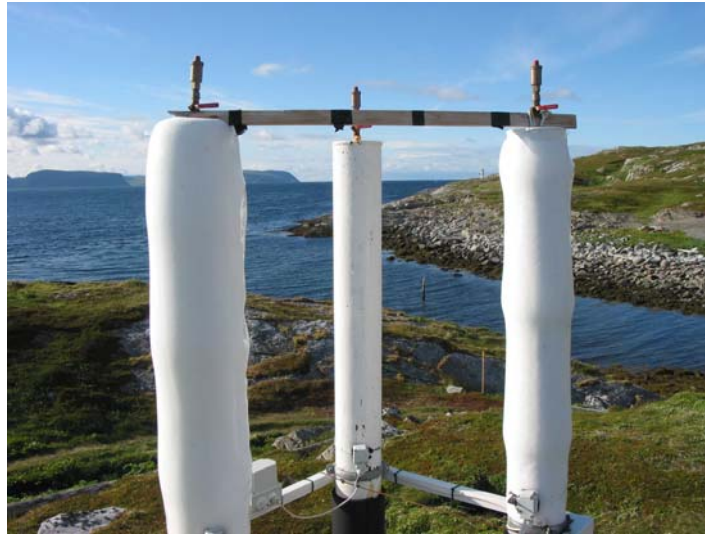
Fig. 6. Riming measurement cylinders at Melkøya, with surface temperatures -15^{\circ}\text{C} (left cylinder), 5^{\circ}\text{C} lower than ambient air temp. (middle cylinder), and -5^{\circ}\text{C} (right cylinder).
