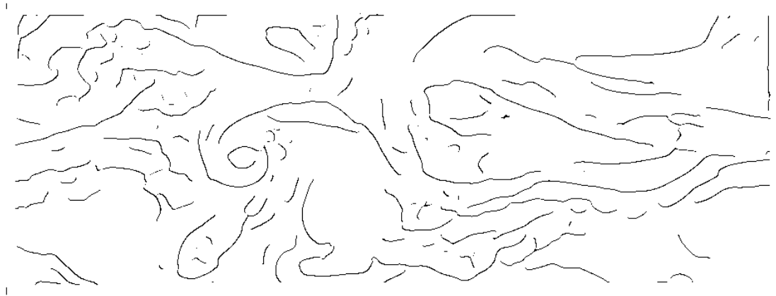
Figure 14: Result of edge detection with lower kernel size for blurring. HT 3, LT 2, KS 5.
