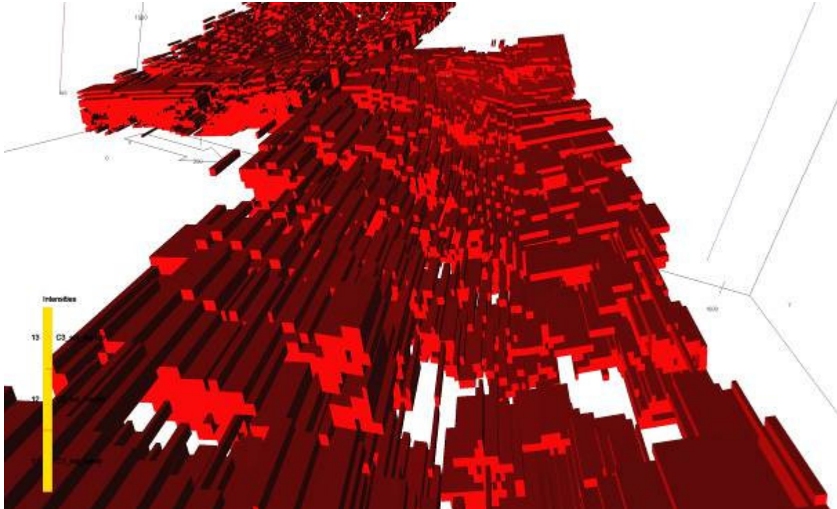
Figure 4.3.2 Visual inspection 2-500mD fault plane perpendicular permeability.
