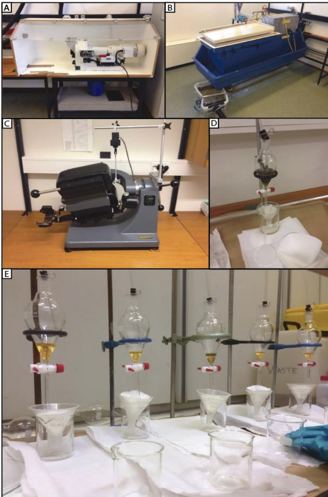
Fig. 4.2: Overview of the steps during the mineral separation. A: Fritsch Pulverisette 13 discmill. B: Holman-Wilfley shaking table. C: Frantz Magnetic Separator. D: LST (Low toxicity Sodium Heteropolytungstates). E: DIM (Di-Iodomethane)
