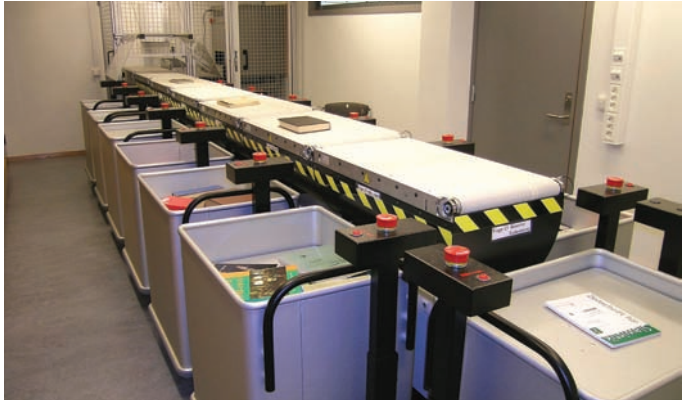
Right: Behind the wall. Transportation line with automatic sorting of books.
