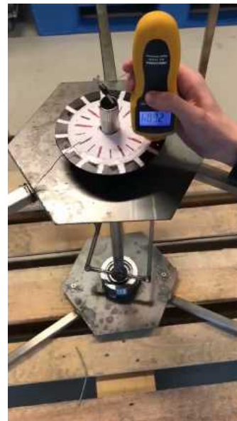
Figure 6: Measuring the RPM of the Column.
