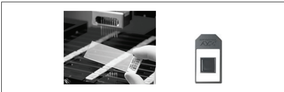
Figure 6: Two common types of microarrays. A custom cDNA array printed on glass (left) and an Affymetrix Genechip ® (right).
