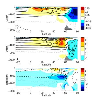
**Figure 4.3:** Upper panel: Shading: Anomaly of the zonally averaged Atlantic salinity for  $\alpha = 2$  in PSU at t = 250 yr. Contours: Atlantic overturning streamfunction for  $\alpha = 2$  at the same time; dotted is zero contour, solid is positive. Contour interval 2 Sv.
