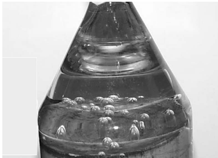
Fig. 14. Oil droplets on the core surface during spontaneous brine imbibition.
