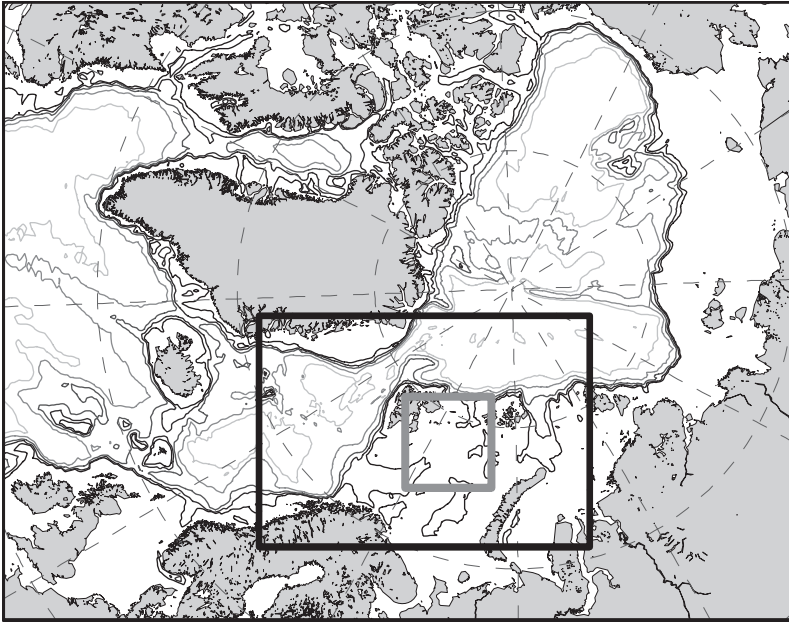
Figure 1. Map of 20 km grid model area. Depth contours at 300, 500, 1000, 2000 and 3000 m. Nested into the 20 km model is the large 4 km grid area (black rectangle) which in turn provides boundary conditions for the main 4 km/800 m model (grey rectangle).
