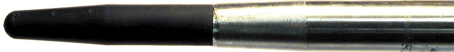
Figure 5.2. Side view of the Reson TC4034 hydrophone mounted in a steel tube.
