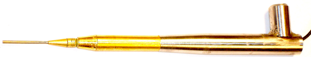
Figure 4.3. Needle hydrophone in horizontal mounting tube.
