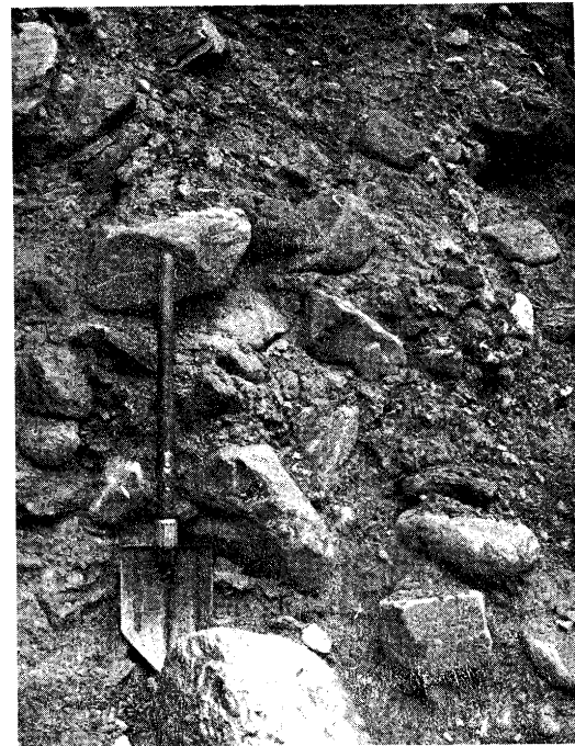
Fig. 12. The uppermost stoney till, B, which is interpreted as an ablation till. The material is coarse and the content of far-transported, often rounded particles is higher than in the basal tills.
