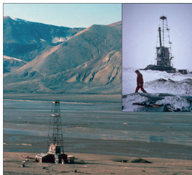
Figure 12. Russian rig in Petuniabukta, Billefjorden, where coal drilling in 1991 resulted in gas blow-outs and small amounts of oil reaching the surface. Photo by Winfried Dallmann, Norwegian Polar Institute, 1993, published by Elvevold (2015). The inset image shows the same borehole in spring conditions, photo from Kjærnet & Elvevold (2012), photographer Torfinn Kjærnet.
