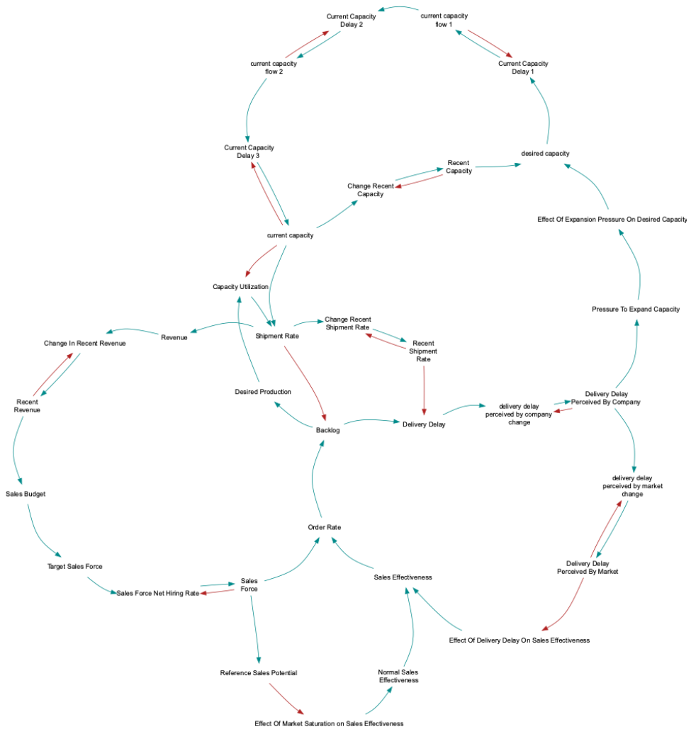
Figure 5: Autogenerated CLD of the full model structure of Forrester's 1968 Market Growth model showing the ability of the edge curving algorithm to generate CLDs which emphasize the loops. Reproduced directly from Article #2.
