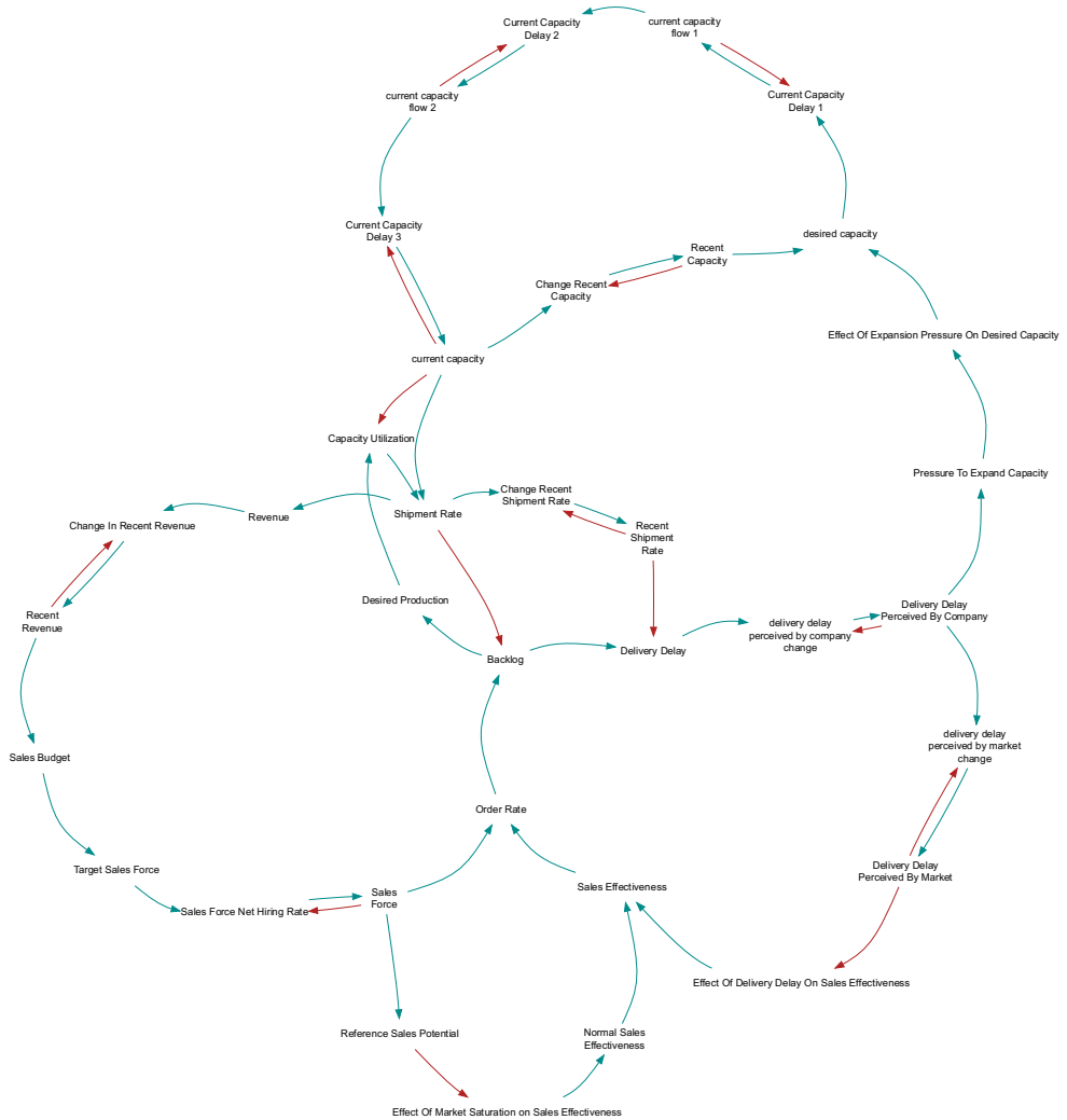
Figure 4: Autogenerated full CLD of Forrester's 1968 market growth model (link inclusion threshold 0%, loop inclusion threshold 0%.) Red links are negative, green links are positive.
