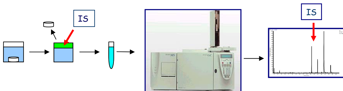
Figure 8. Specimen immersed in ethanol. After 24 hours the specimen was removed and IS added. The sample was concentrated and injected in the GC-MS. Eluted substances were separated and recorded.
