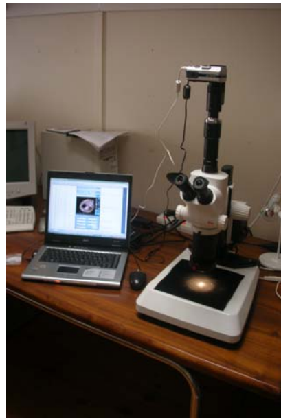
Fig. 4.1 (left). Initial analyses with a Nikon microscope. Fig. 4.2 (right) final analyses using a Lecia S8AP0 microscope equipped with a Canon digital camera attached to a computer (Photographs by T. Kjosvold and I. Vibe).
