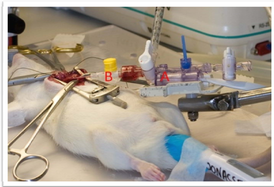
Figure 12. Pressure measurement setup. A fluid filled pressure transducer (A) was connected to a 25G i.v. cannula, used as a pressure catheter (B), placed into the right ventricle of the rat heart for pressure measurement.
