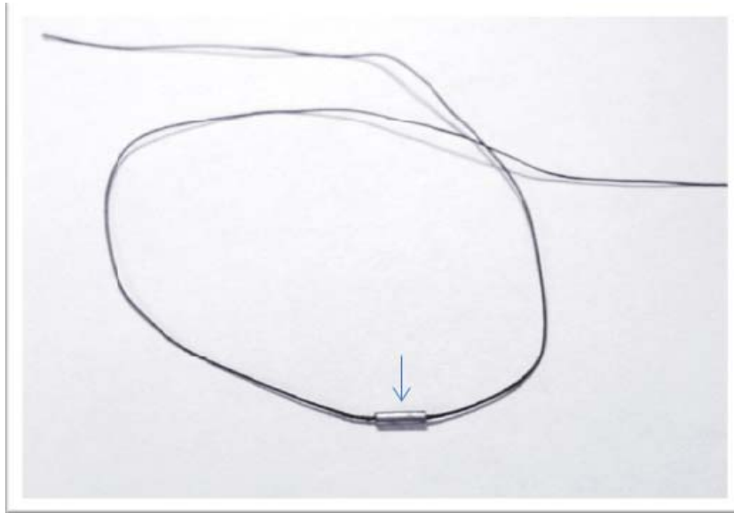
Figure 10. Luer stub adapter. A 16G luer stub adapter was used to produce a pulmonary artery (PA) banding of the same diameter in each rat. For practical reasons, the small adapter was threaded onto a suture and knot in both ends of the adapter.
