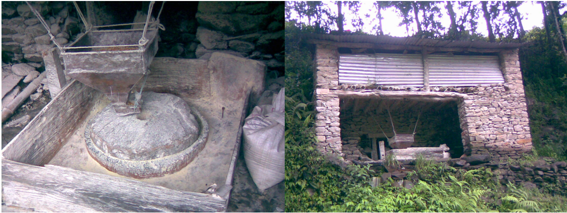
Traditional Grinding Mill is used for the Livelihood of Rural Communities in Nepal.
