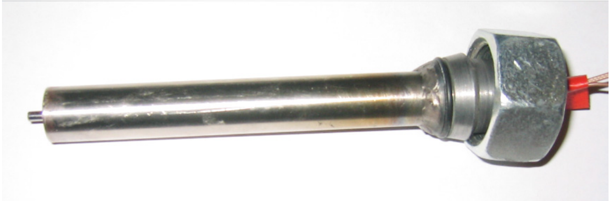
Figure 4-4 The ionisation probe used in some preliminary experiments in the 20-litre vessel.
