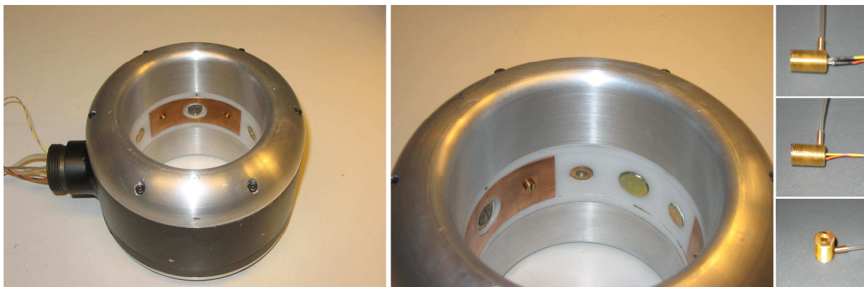
Figure 3-10 Optical/impedance probe for monitoring gas and dust explosions(left) and measure-heads (right).
