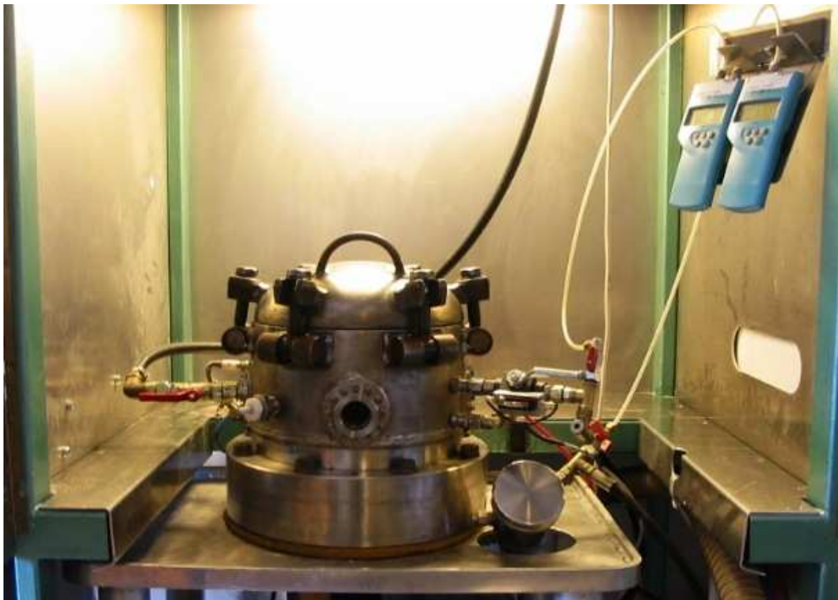
Figure 3-2 20-litre explosion vessel situated at the dust-explosion laboratory at the UiB. The two blue displays in the upper right corner are the digital pressure indicators for controlling the pressure in the vessel and dust reservoir pressure.
