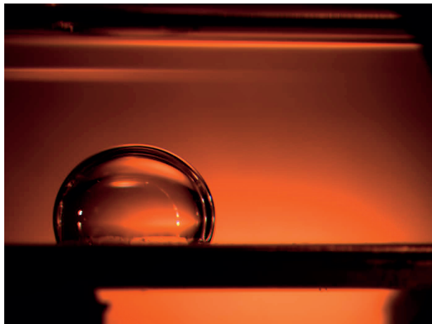
Figure 3.2: Oil-wet system: A water (buffer) drop resting on a brass surface in model oil (petroleum ether). Picture acquired during laboratory experiments by the author.
