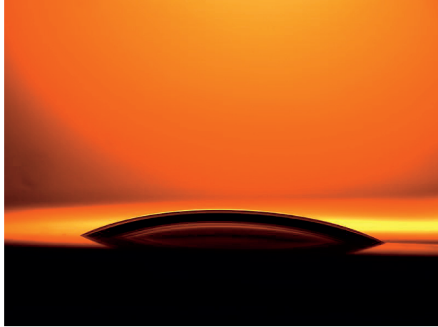
Figure 3.1: Water-wet system: A water (buffer) drop resting on a glass surface in model oil (petroleum ether). Picture acquired during laboratory experiments by the author.
