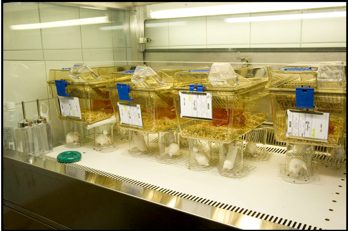
Figure 6) Urine collection for the screening for glucosuria in mice. The procedure is carried out in a laminar flow hood.
