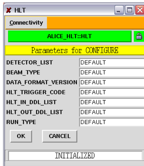
Figure B.1: Screenshot of the ECS test-GUI, showing the HLT in INITIALIZED state and preparing a CONFIGURE command plus parameters to be sent.
