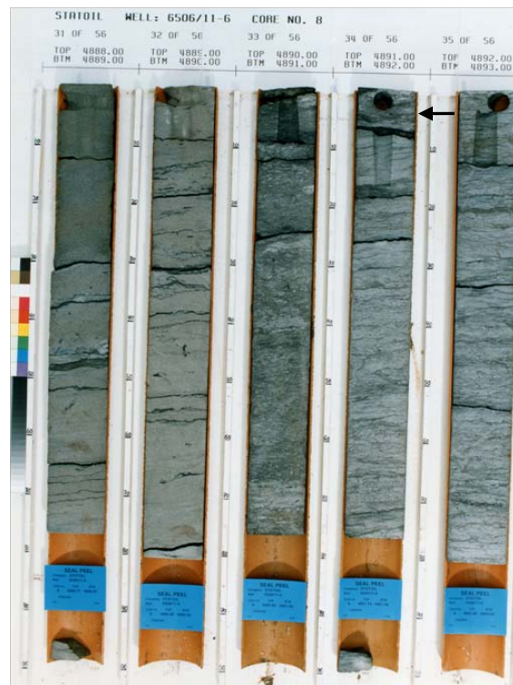
Figure 5.3: Prodelta fines abruptly overlain by mouth bar sands (boundary not seen, but the two core meters on the left are interpreted as mouth bar sands). Black arrow indicates base of sudden fining of prodelta sediments in well 6506/11-6, core depth 4888-4893m (Norwegian Petroleum Directorate web pages, 2010).
