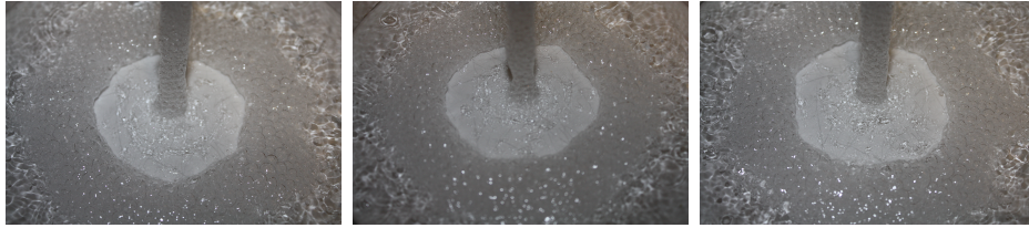
Figure 2.2: Three pictures of a hydraulic jump created by here at University of Bergen by letting water run from the tap down on a flat surface. As the water hits the flat surface it carries a lot of momentum. Shooting out to the sides it obtains a supercritical flow and shortly after preforms a hydraulic jump. The jump is marked by a region of turbulence and beyond this region the surface is calm.
